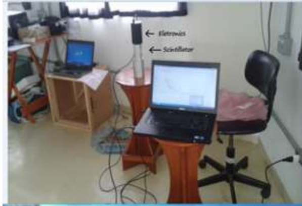
Fig. 1 – Sodium Iodide scintillator ( 3x3 inches) and photomultiplier used in this gamma radiation measurement, (Aware Electronics, INC, USA).
