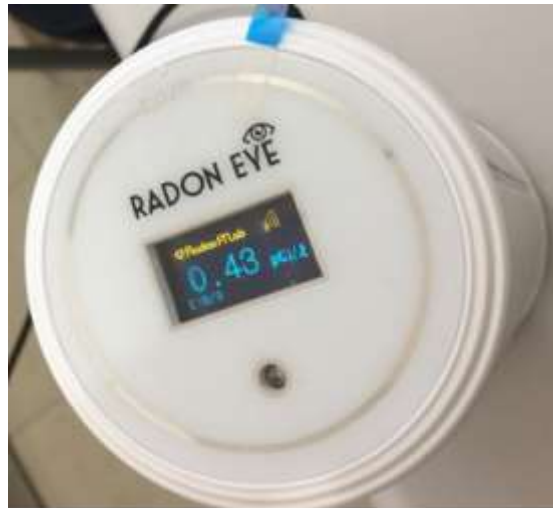
Fig 2 – Top view of Radon Eye RD200 ionization chamber used for monitoring radon gas [7]
